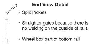
Note: UL 325 requires electronically operated gates and the fence line adjoining such gates to have a maximum 2 1/8" picket spacing or mesh installed. For additional cost, contact sales person.
