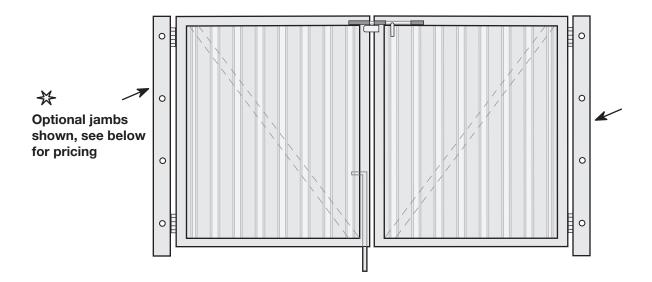
Gates are manufactured with 1/4" x 2" x 2" angle frames, 1/4" x 2" flat bar diagonal bracing, 20 GA galvanized decking, factory installed 4 x 4 butt hinges, heavy drop rod and slide bolt. Gates are shipped with one coat high solids primer only.
